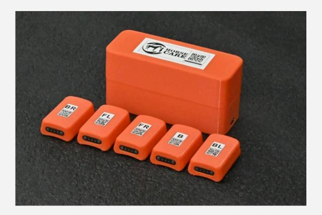
The sensors are very durable and will work even if they are thrown into sand, submerged in water, or lightly hit with a hammer. They require power to operate, so they have a battery inside. For recharging, a special cradle is provided, which immediately serves as a convenient storage case. The sensors start functioning when you remove them from the cradle, and turn off when you put them back.
