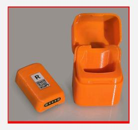
The rider sensor must be attached to the body (body) of the rider and is designed to collect data about the movement of the rider on the horse. In the future, riders, after analyzing the data received from this sensor, can make adjustments to their behavior on the horse during training, thereby improving overall training performance.
